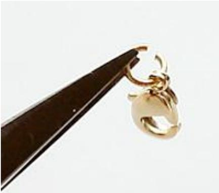
7.) Connect the end of the bracelet to the jump ring; then close the opening with the pliers.
