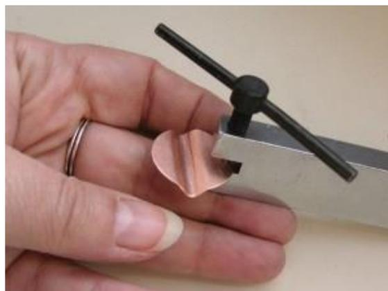
5.) Lay the disc onto the forming block, laying the crease into a valley, as shown. Use the center punch to create a pattern (you can mark the pattern on the disc with a Sharpie). One method is to file the tip of your punch, and punch on the BACK, so that the pattern is in relief on the front, but you can create the
