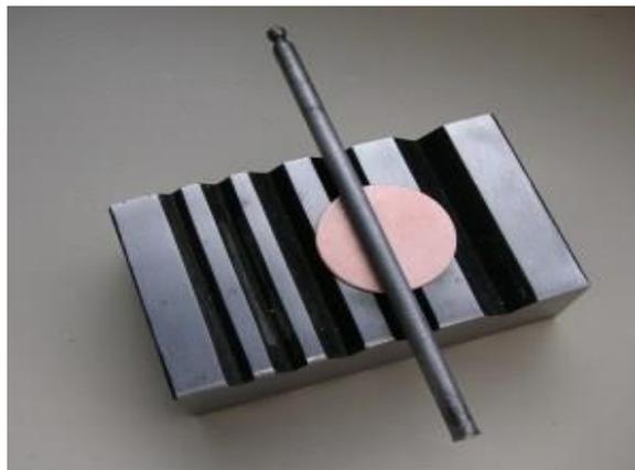
2.) Hold the punch firmly in place, and hammer it on the disc, into the valley, forming the metal (repeat to get a good crease).
