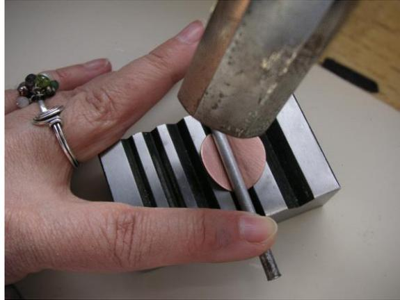
3.) Remove the punch, and flatten the disc edges using a wood or rawhide mallet. If you don't have a mallet, lay a piece of leather over the disc, and use the hammer.
