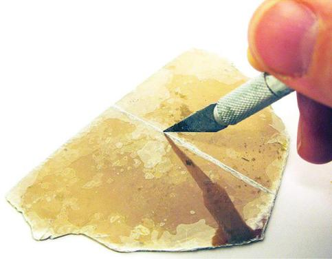
2.) Once you have a piece of mica in the shape you want you will need to split it into two identical pieces. Fit the tip of your craft knife in between the layers of mica and gently split the layers by twisting the knife sideways until you have two pieces. If the edges of the mica seem like they will continue to split you can put a thin layer of Diamond Glaze on the edge with a paintbrush or your fingertip. Allow the glaze to dry at least 20 minutes before continuing.
