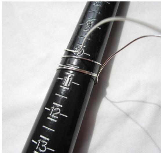
3. After step 2, the ends of the wire should end up in the front. Gather all the wires closely together and move them to about a 1/2 size bigger than the ring size you are trying to make.
