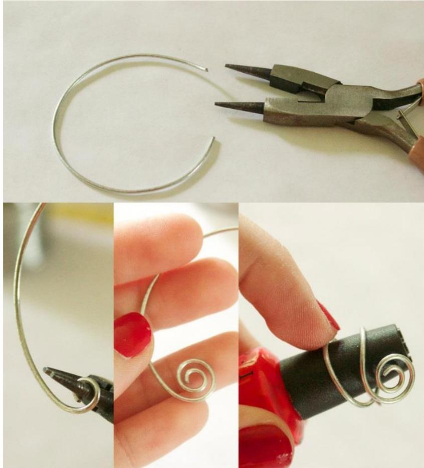
3. Make a small loop at the end to finish the end. If you need to trim your wire beforehand to make it the appropriate length, do this before looping.
