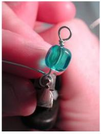
20.) Before wrapping your loop, slide your previously wrapped headpin onto the eye. Then, grasp across the flat area of the eye loop, wrap end around shank of eye pin, cut your excess wire, and flatten your end.
