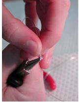
2.) Flatten this loop closed against itself with your needle nose pliers. You may need to start at the bend in the loop and work in towards the end to get it nice and tight. This is going to create the beginning of the spiral base that will be our headpin.
