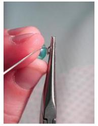
13.) Cut the excess wire from the wrapped coil, pushing the flat back end of the wire as close to the coil as possible.
