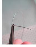
16.) Grasp a small distance from the bend; create your eye loop and wrap loop as before. Cut away any extra wire.
